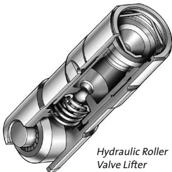
Hydraulic Roller Valve Lifter
